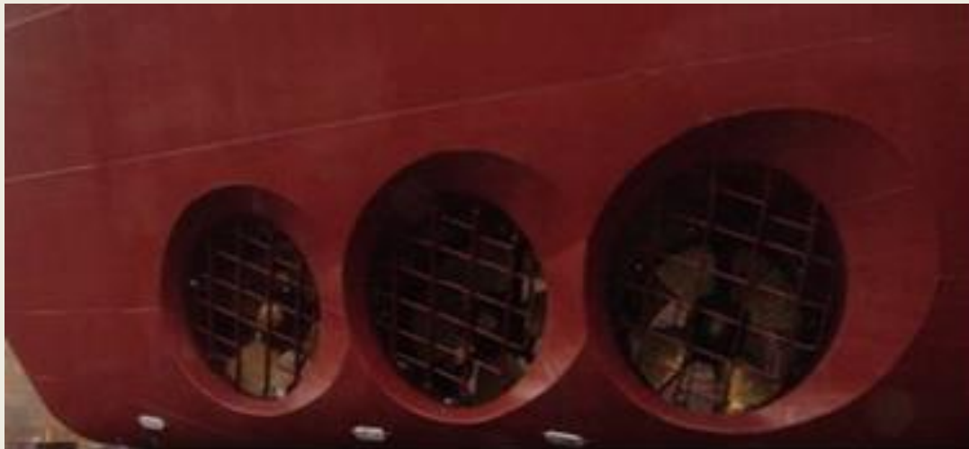
Examples of tunnel thrusters with conical inlet. (Photo: Brunvoll )
